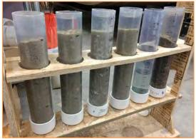
Figure 4-27 Spent Lime/Sand Mixture Column Testing
