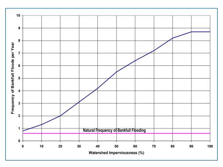
Figure 4-8 Conceptual Frequency of Bankfull Flooding as a Function of Imperviousness (9)
