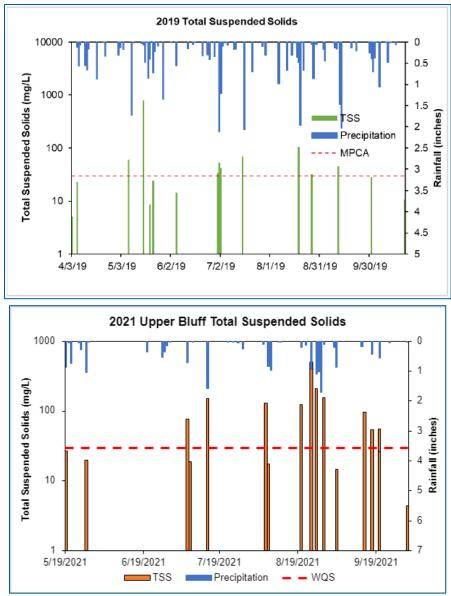
Figure 4-5 Bluff Creek TSS Measurements at Galpin Boulevard (2019 above and 2021 below)
