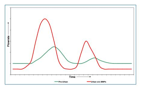
Figure 4-7 Example change in Streamflow Due to Urbanization (9). Note this is a general example, not based on flow data from Bluff Creek
