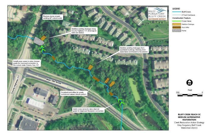
Figure 5-8 Concept B: Moderate Concept Restoration of Reach B5C
