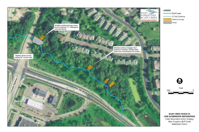
Figure 5-5 Concept A: Low Concept Restoration of Reach B5C
