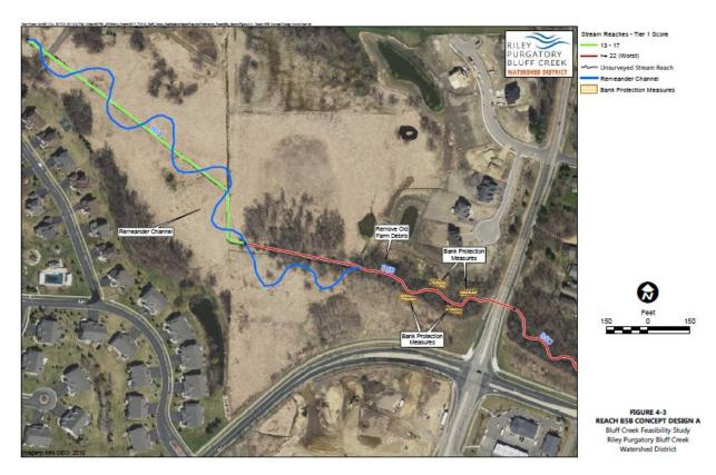
Figure 5-3 Concept A: Restoration of Reach B5B by Remeandering
