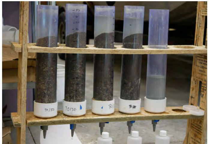
Figure 58. Column testing for lime/sand mixture.
