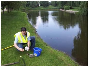
Figure 5. Filtering the water samples through the 1.5mm mesh filter.
