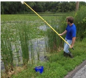
Figure 4. Using the sampling stick to collect the composite water sample.
