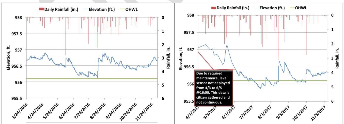
Figure A-6. **Lake Lucy** level elevation data (ft.) for 2016 and 2017 along with the lake's ordinary high-water level (OHWL). Daily rainfall (in.) is displayed along the top of the graph (NOAA).
