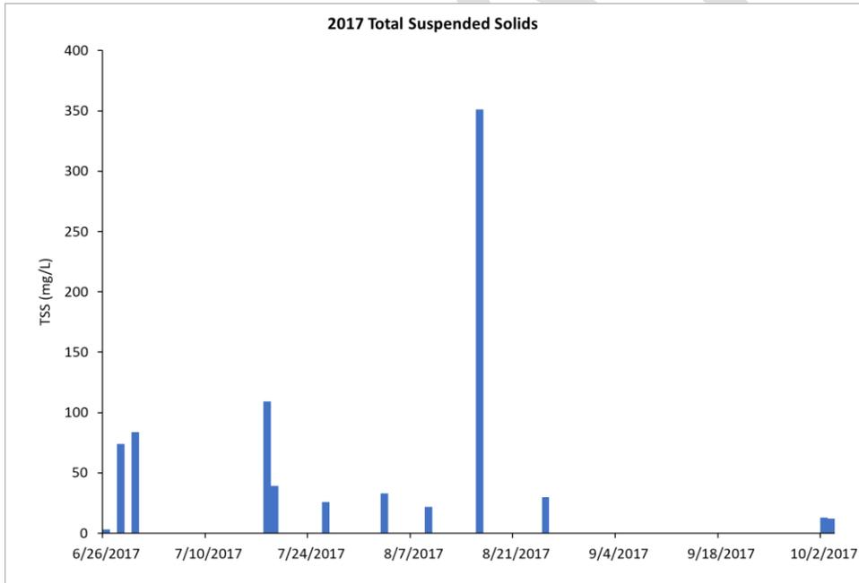
**Figure 4.10-3 2017 Stormwater Total Suspended Solids Input to Rice Marsh Lake**
