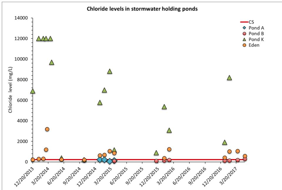
**Figure 4.5-2 2013-2017 Chloride Levels within Stormwater Ponds**
