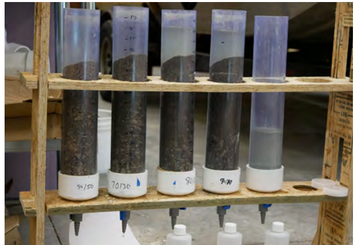
Figure 58. Column testing for lime/sand mixture.
