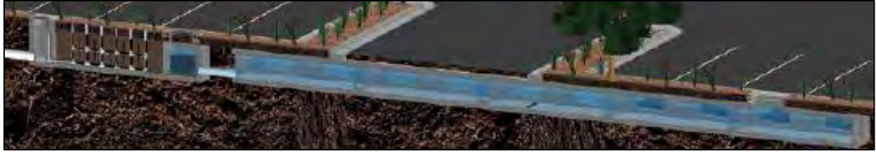
Schematic of Modular Wetland System – Linear with upstream underground storage vault (BioClean Environmental, 2015).
